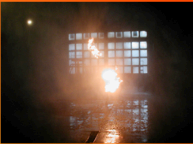
Above is 6.0MW Diesel spray fire getting extinguished within 12 seconds from Fogex system activation.
